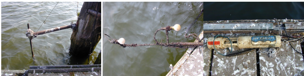
Pict.6: Boom with PAR sensors; Pict.7+8: typical plant growth on the PAR sensors and multi-parameter sensors
